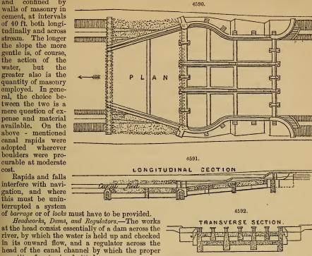
quantity of water is admitted. In most cases the canal is taken out of a branch of the main river, and the permanent dam is thrown across the branch only, the water being diverted from the main stream into the branch by temporary dams constructed of boulders, which are swept away on the rise of the river, and are annually replaced.
